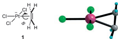
Figure 1. Crystal structure of the complex anion of Zeise's salt ( 1 ) together with a schematic representation.
